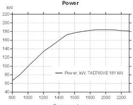
Engine speed, rpm
